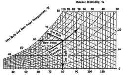
and humidity has been codified in a diagram called the psychrometric chart that is indispensable for understanding condensation. A psychrometer or hygrometer is used to measure the water vapor content in the atmosphere or humidity. The first crude device was invented by Leonardo Da Vinci in the late 1400's.
